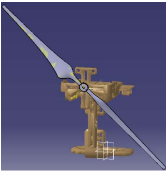
Figure 1: Improved propeller design created by Inholland student on a testing mount (left) and 3D render (right).
