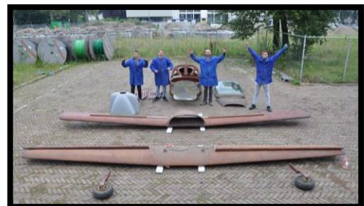
Besides manufacturing new components, modifications on the airplane its primary structure shall be performed. The DragonFly is going to fly using electric propulsion to lower the carbon emissions in the industry. Hence, the structure shall be modified to implement batteries as a power source for the electric motor. The structural integrity must always be taken into account while designing and implementing structural modifications to guarantee safe flights.
